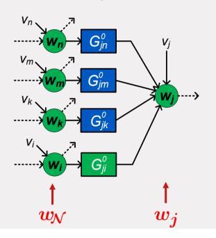
Multi-input single-output identification problem addressed by either a direct or indirect method
